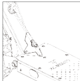
A) The charging port is in the front of the footboard with a cover.
