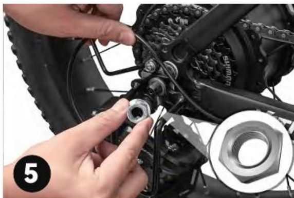
Step 5: Putting the bolt on the axle.
