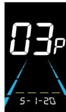
Figure 6-4 PAS level setting interface
