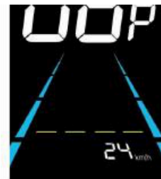
Figure 6-7 Speed limit setting interface
