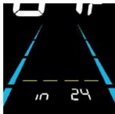
Figure 6-5 Wheel diameter setting interface
