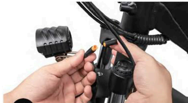
Pasul 4: Aliniați the arrow on the headlight connector and connect it to the cable connector.
