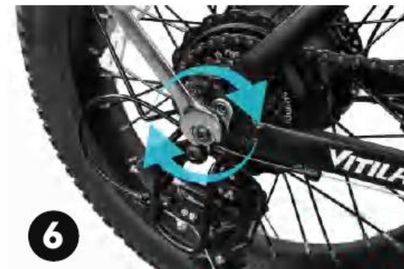
Step 6: Using an 18mm wrench to fasten bolt several times clockwise.
