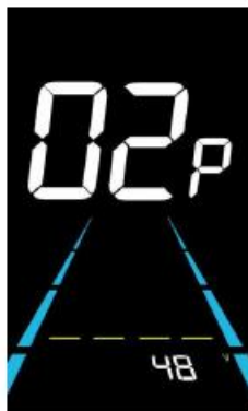
Figure 6-2 Rated voltage setting interface
