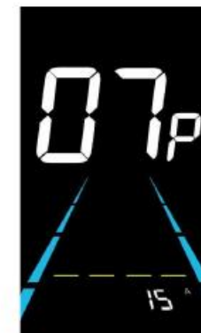
Figure 6-8 Controller current limit setting interface
