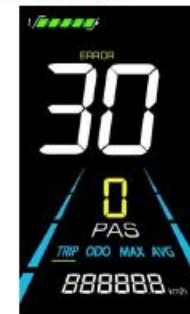
Figure 5-5 Error Code Display
