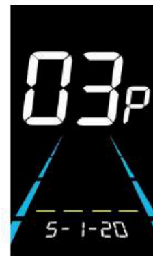
Figure 6-4 PAS level setting interface
