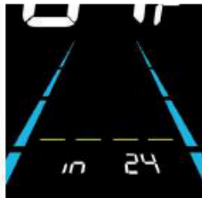
Figure 6-5 Wheel diameter setting interface
