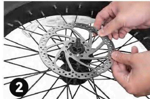
Krok 2: Vyrovnějte its 6 holes with the 6 holes on the hub.
