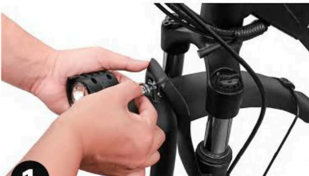
Pasul 1: Montați the headlight, bolt and spacer through the headlight mounting holes, spacer and front fender hole.
