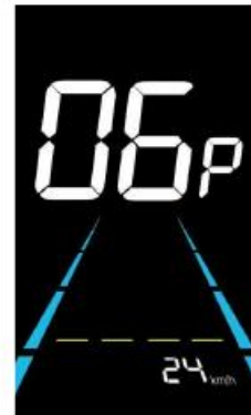
Figure 6-7 Speed limit setting interface
