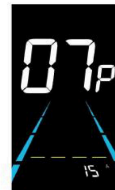
Figure 6-8 Controller current limit setting interface
