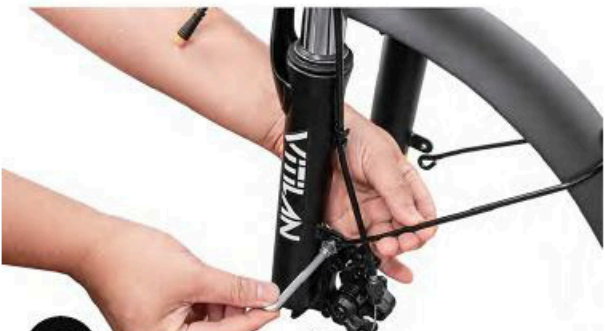
Pasul 3: Bolt the left and right front-fender brackets to the front fork.
