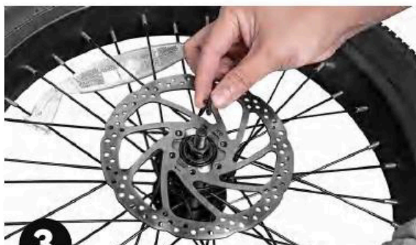
Krok 3: Vložte the 6 brake screws.
