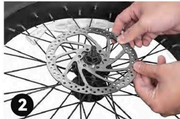
Pasul 2: Aliniați its 6 holes with the 6 holes on the hub.
