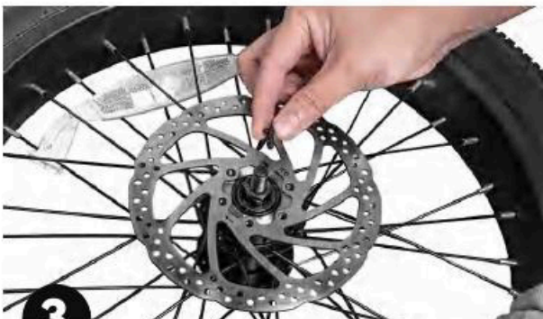
Pasul 3: Introduceți the 6 brake screws.
