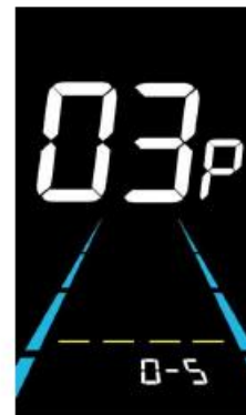
Figure 6-3 PAS level setting interface
