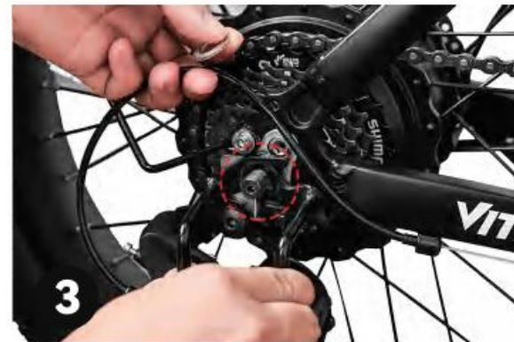
Step 3: putting the rear derailleur guard on the rear wheel axle.
