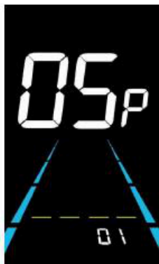
Figure 6-6 Number of speed sensor magnets setting interface
