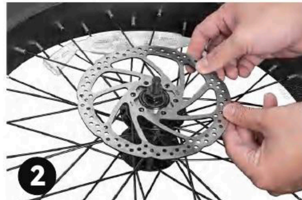
Lépés 2: Igazítsa its 6 holes with the 6 holes on the hub.
