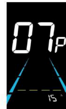
Figure 6-8 Controller current limit setting interface
