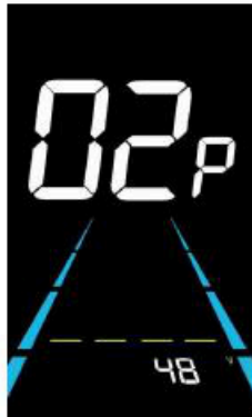
Figure 6-2 Rated voltage setting interface
