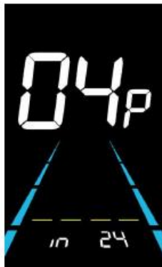
Figure 6-5 Wheel diameter setting interface
