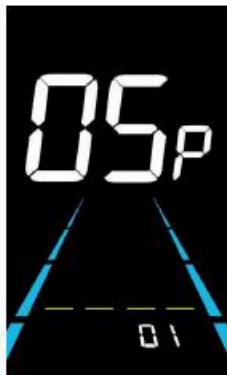
Figure 6-6 Number of speed sensor magnets setting interface
