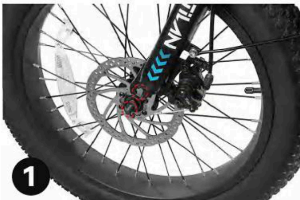
Pasul 1: Aliniați the roata față and axle, then insert the axle into the front fork.
