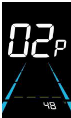
Figure 6-2 Rated voltage setting interface
