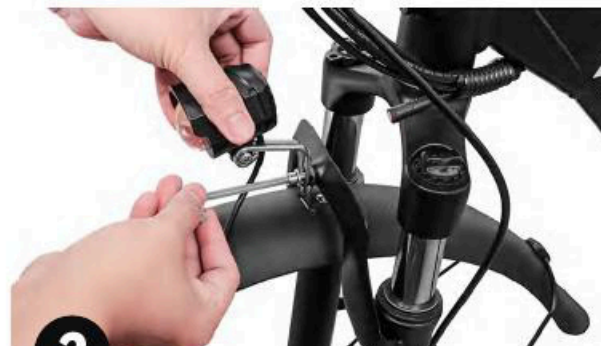
Pasul 2: Center the headlight and tighten the nut with a 5mm cheie hexagonală.
