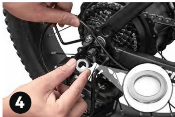
Step 4: Installing the spacer on the axle.
