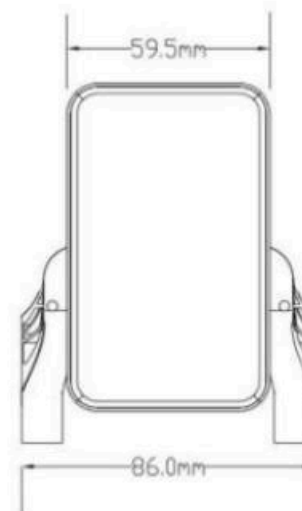
Figure 3-3 YL-81F Front View Dimension
