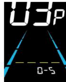
Figure 6-3 PAS level setting interface
