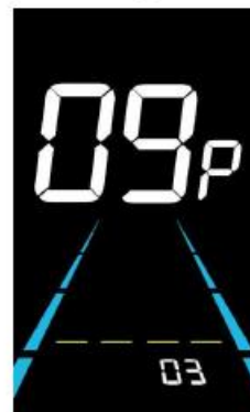
Figure 6-10 Pedal assist sensitivity setting interface
